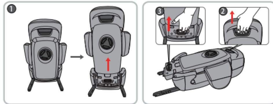
FOLD CAR SEAT :lift headrest till the fold button be exposed by pull headrest adjusting button.pull fold button to fold backrest .withdraw back headrest the headrest till the limit.
